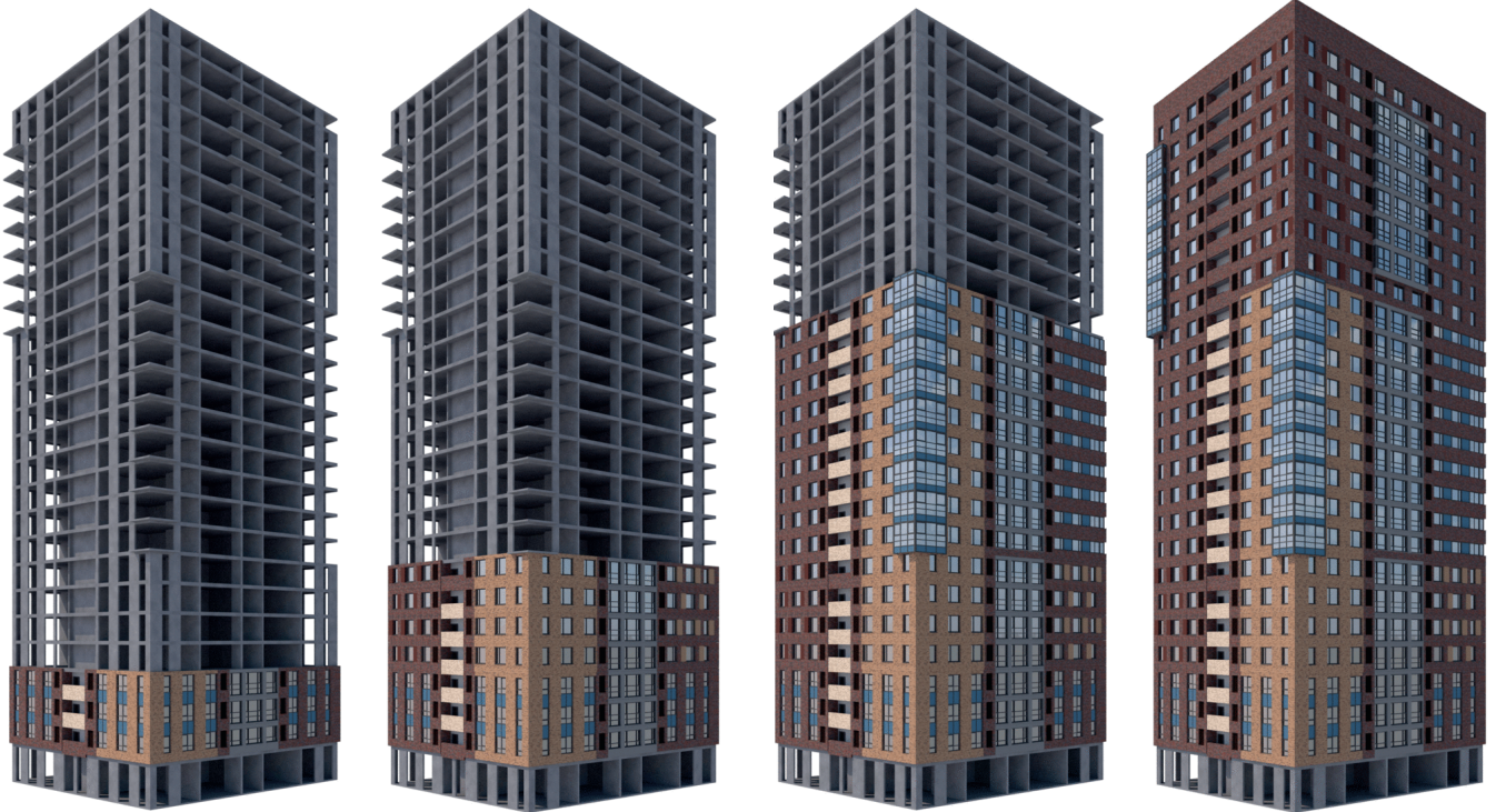
4 façade sections of repetitive module panels
