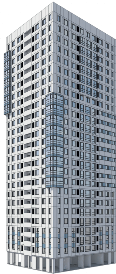
The façade divided into sections of repetitive module panels
