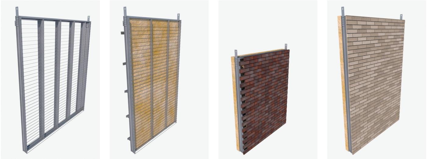
Wall panel structure and different wall panel types, all in one GDL element
